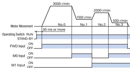
● When operating in 4-speed settings, the rotation direction of the motor cannot be changed by external input signals. (Only for 30 W, 60 W and 120 W)
